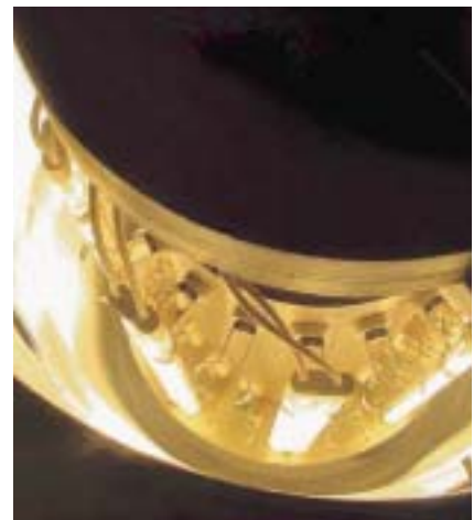
Interior heating of compressor housings
